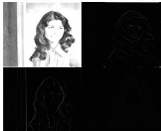
Fig. 2 An one level 2-D DWT decomposition of Woman image (LL, LH, HL, and HH=128x128)
