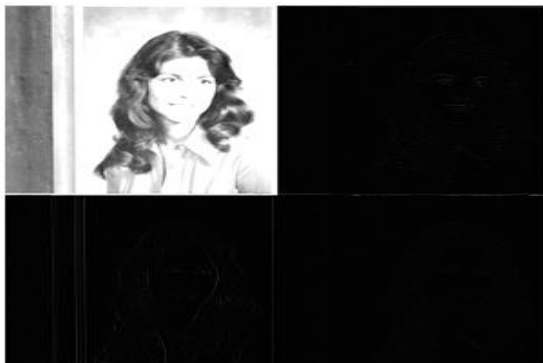
Fig.4 The process of 1 level 2-D RDWT decomposition process (LL, LH, HL, and HH =256x256)
